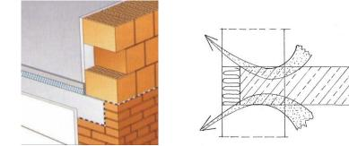
Fig. 3. Thermal bridges in a single-layer wall with a poorly insulated reinforced concrete tie beam
