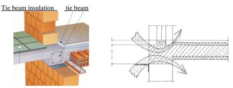
Fig. 4. Thermal bridges at the connection of the floor with a cantilevered balcony. The corners where the floor-wall meets lose heat (freezing effect - the occurrence of mold and mildew)
