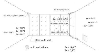
Fig. 6. Air temperature  $\Theta_i$  and wall surface temperature  $\Theta_{si}$  are at the expected level. In the corners, the temperature  $\Theta_{sin}$  is a few degrees lower. Residues of mold appear in these areas
